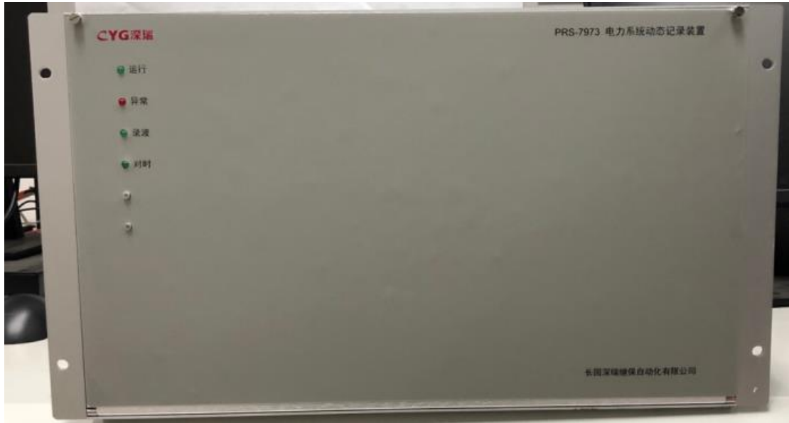
Figure 3-1 Power system dynamic recording device face-up diagram
