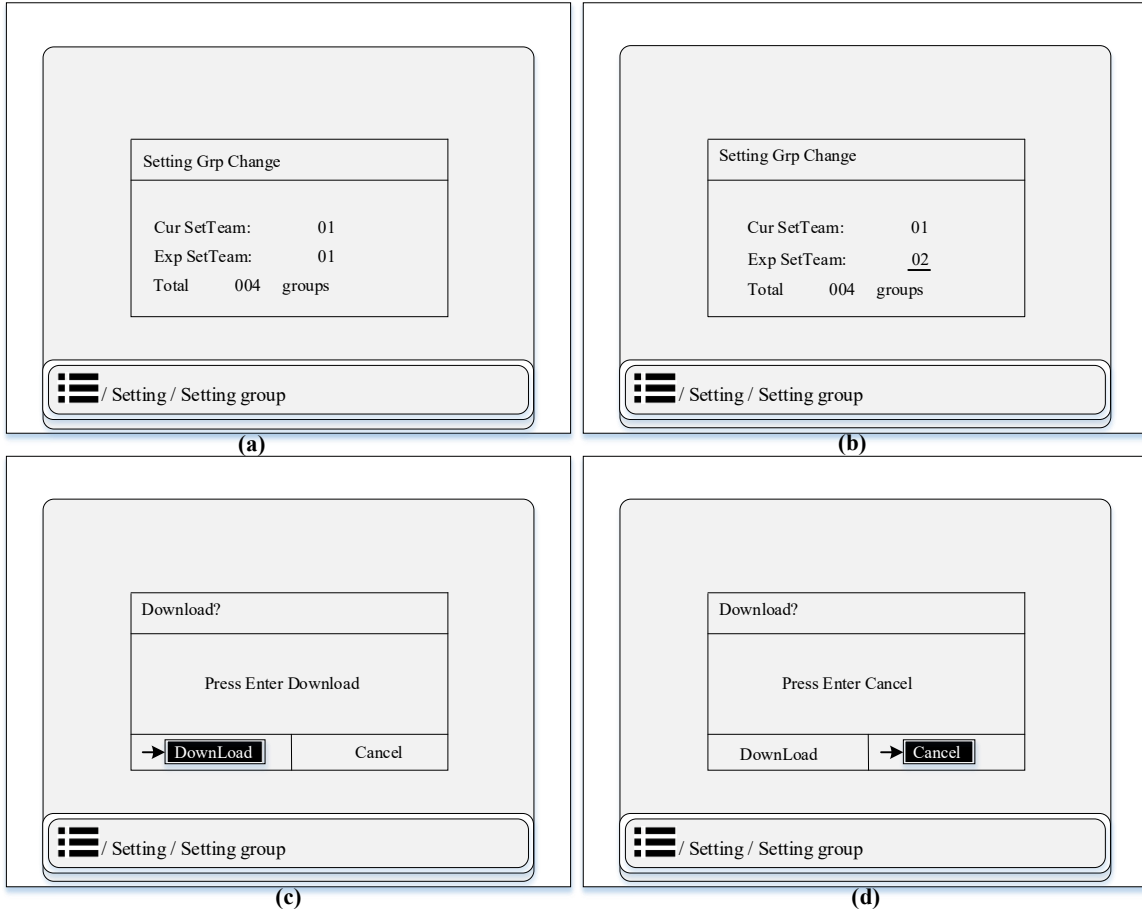
Figure 7.3.21 Procedure Diagram of Group Setting Change
