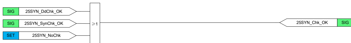
Figure 3.30.5 Logic diagram of Synchronism Output
