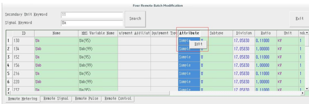
Figure 3.2.64 Batch Modification of Four-remote Attribute Based on Keywords
