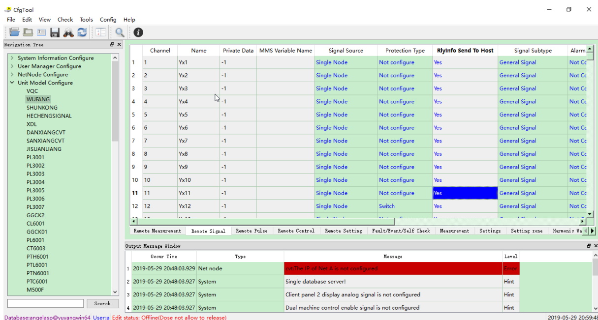
Figure 3.2.90 Interlocking Signal Mapping of SCD Virtual Terminal
